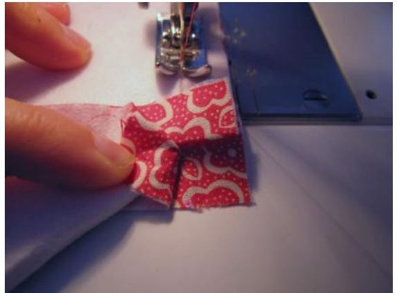
Starting at the very top (after unfolding the folded edge) stitch along the marked line, sewing two sides together. As you approach the bottom, fold the seam allowance from the bottom square out of the way as shown above.
